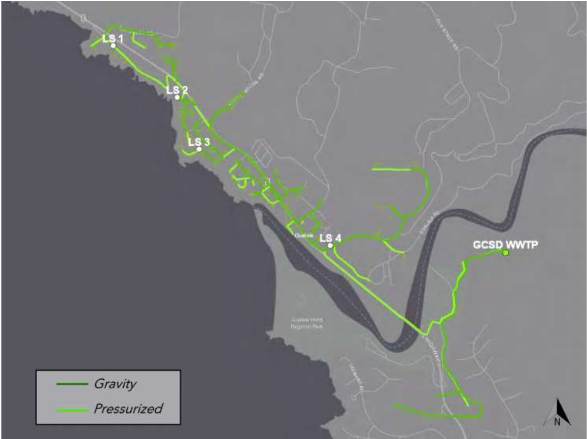
Figure 3-4 GCSD gravity and pressurized sewer mains
