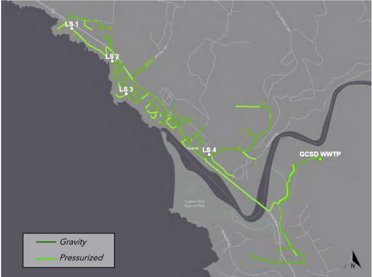
Figure 3-4: GCSO Gravity and Pressurized Sewer Mains
